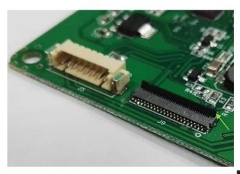
Then plug in the DSI Cable, make sure the contacts are on the TOP side
