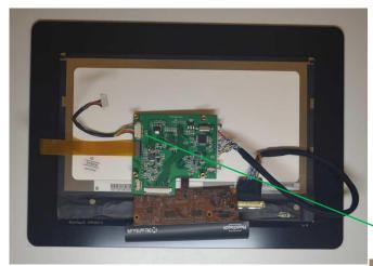
The USB Cable will look like this picture And then you can fix the 4 spacer with the 4 nuts Plug in the USB bridge Cable on the 10 pin side on the DSI board
