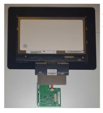
Bring the Display with touch and align from back side with the DSI converter board, open the 4 PINS ZIF connector on the DSI board
