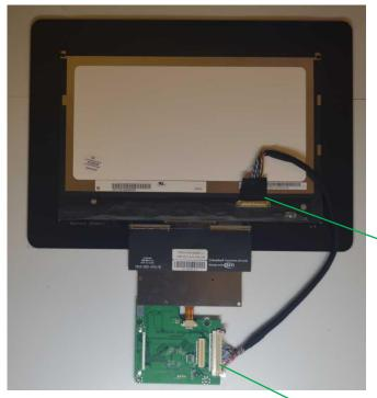
After you plug in the 4 pins Touch FPC into the 4 pins ZIF connector, then bring the LVDS Cable and plug in the white connector side on DSI converter board then the Golden side on the Display Connector, make sure the side is correct and is all plug in
